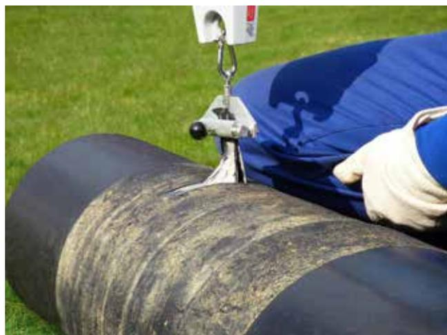
Figure 4. Cohesive separation pattern after 39 years.
