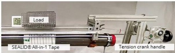
Test setup - Overview
