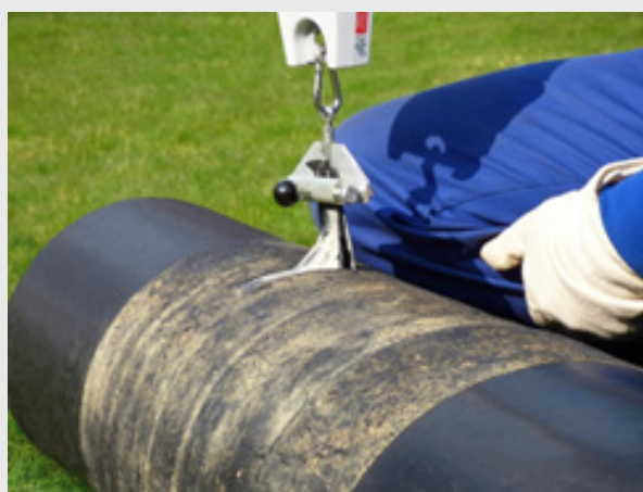
Figure 9: Cohesive separation pattern after 39 years
