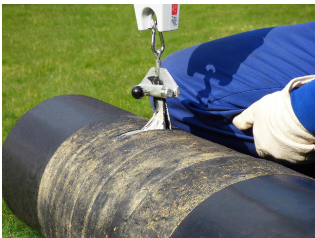
Figure 4. Cohesive separation pattern after 39 years.
