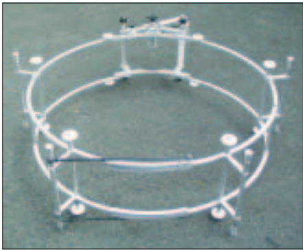
Fig. 3: cage-DENSOMAT KGR Junior with low weight aluminium frame
