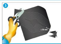
■ DEXPAND®-DRP is cut to size so that there is a minimum overlap of 50 mm on all sides of the undamaged factory coating. The corner areas must be rounded off.
