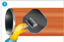
Press on **DEXPAND®-DRP** with a hand roller in longitudinal and circumferential direction smoothly and bubble-free until the adhesive coating emerges visibly on all sides.
