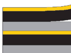
Fig. 9: Delamination effect during peel-test
