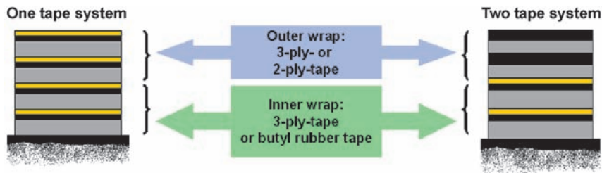
Fig. 7: Cross sectional view of a one tape and a two tape system
