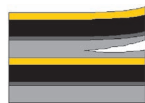
Fig. 10: Cohesive peel mode by co-extruded intermediate layer of high-performance tape
